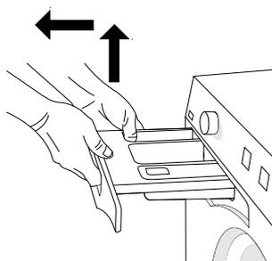
Rinse the compartment and scrub it clean. The fabric softener compartment cover can be removed.
