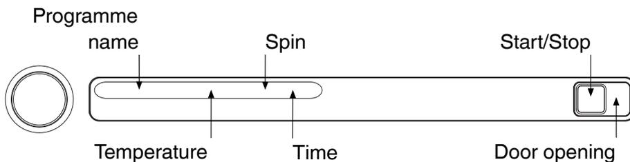
The display shows the programme name, the water temperature and the spin speed.
