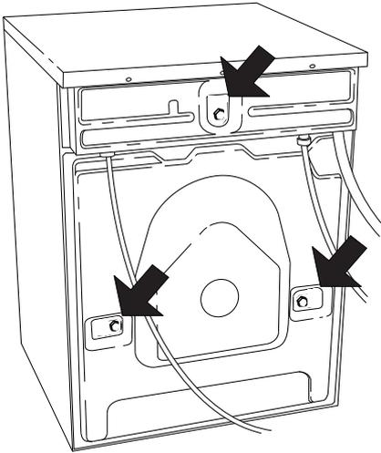
1. Loosen and remove the screws.
