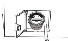
4. Turn the cover anti-clockwise to open the pump. Remove the cover.
