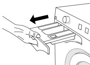
Lift the detergent compartment upwards and then outwards to remove it from the machine.
