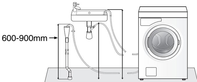
The machine can also be connected to the drain via a spigot connection. In this case the hose should also be 600-900 mm above the floor. The internal diameter of the hole should be at least 18 mm.
