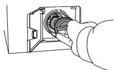
5. Remove any items and so forth from the pump housing and the cover. Also check that the pump blades right at the back rotate.
