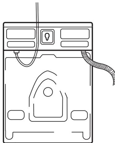
Use only the supply hose supplied with the machine. Do not re-use old hoses or other loose supply hoses.
