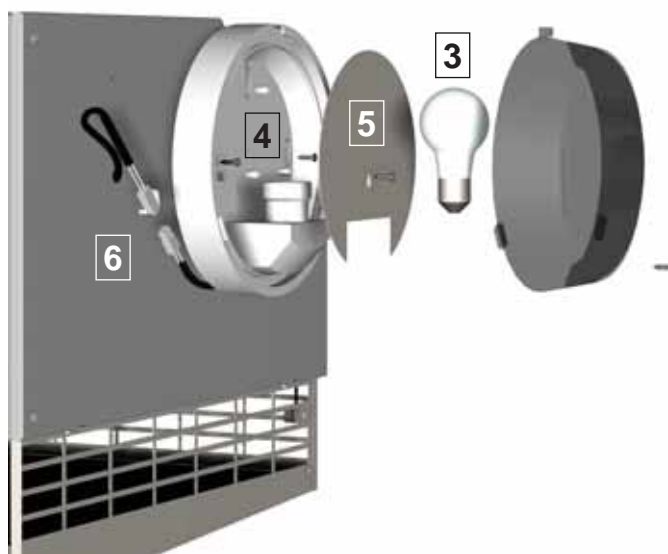
Picture 11b. Mounting of the lamp
