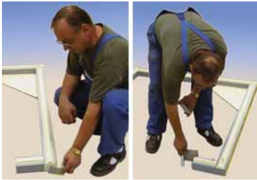
Pic 5. Corner angle plates
