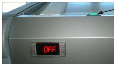
First, push the interrupter and will start to work the fans and the digital controller. This interrupter is above of the digital controller.
