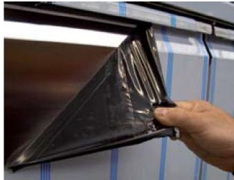
Before starting-up and placing any food inside the cabinet, firstly remove the protective film and then clean the complete unit thoroughly. If any adhesive remains, eliminate it with alcohol. Washing with a mild soap and warm water solution is recommended for cleaning all the stainless steel surfaces of your cabinet. This should be followed by cleaning with a baking soda solution. Rinse thoroughly with clear water and dry with a clean, soft cloth.
