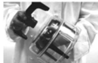
Rotate the knife (B4) clockwise and remove the knife and lift off the bowl. If the contents of the bowl are liquid, it should be emptied before the knife is removed.
