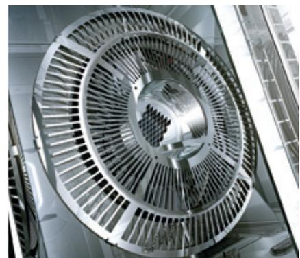
The heat is always optimally distributed thanks to the specific cooking cabinet geometry and the powerful, energy-saving fan impeller drive, which intelligently adjusts the rotation direction and speed to the relevant food product. This ensures excellent food quality even with full loads.
