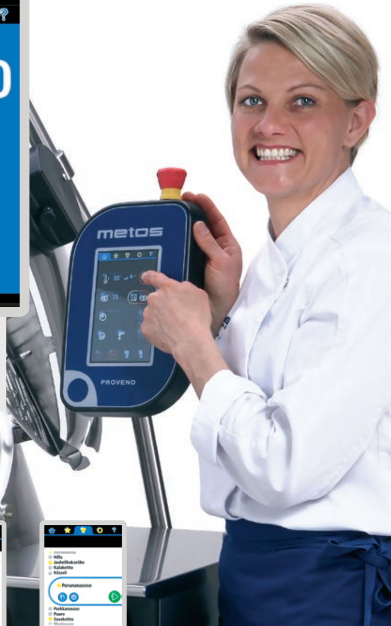
Various phases are displayed on the status display. Audible signals inform the user about any required actions.
