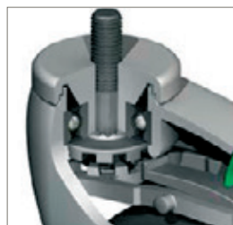
Labyrinth structure protecting the swivel bearing.
