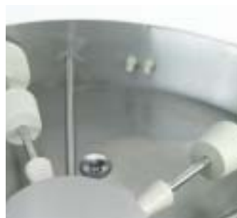
Drain in the bottom of the basin.
