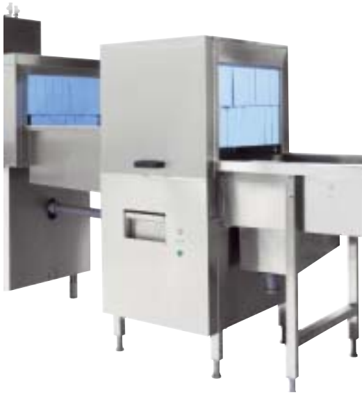
The conveyor from the Nordieflex sorting unit takes the basket to the pre-wash machine and then further to the rack conveyor machine.
