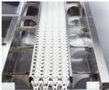
Thanks to the open chain construction cleaning is possible without brushing or lifting up the conveyor. The supports for the conveyor don't block the cleaning way to the basin. The bottom of the basin is sloped towards the strainer.
