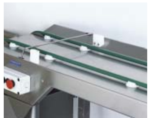
There is a detector placed in the end of the conveyor to make sure no dishes remain on the tray before stacking. Unnecessary breakage of dishes can thus be avoided.
