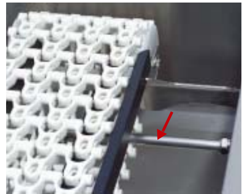
To further guarantee the chain hygiene Metos units have a chain rinsing function as standard. The function can be used either by manual (standard) opening and closing the valve or having it timer controlled (option). Cleaning the chain is easy as the dirt remains loose due to rinsing.
