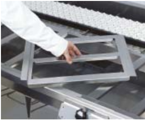
The detachable basket grids can be washed in the dishwasher.
