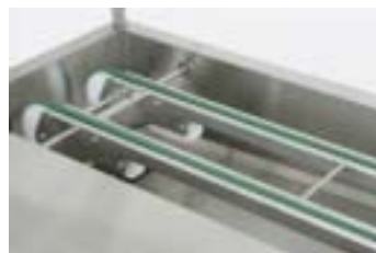
The double round polycord conveyor is almost soundless and easy to clean.
