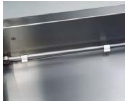
In order to guarantee hygiene in the basin Metos units have the basin rinsing function as standard. The function can be used either by manual (standard) opening and closing the valve or having it timer controlled (option). The food remains dripping from the dishes are thus rinsed already during normal use towards the bottom of the basin and to the strainer. The tidiness of the unit and prevention of unpleasant smells is well under control in Metos units.
