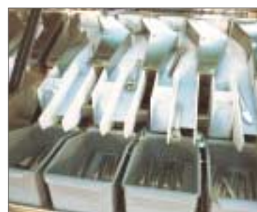
The automatic cutlery sorter distributes cutlery automatically into the correct cutlery boxes which are then transported back to distribution.
