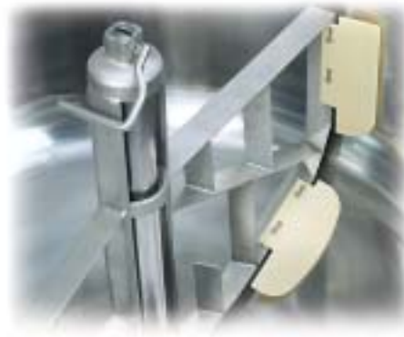
The scrapers of the mixing tool have also a quick locking system.
