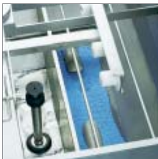
The granules are in a separate basin and are not flushed into the drain.
