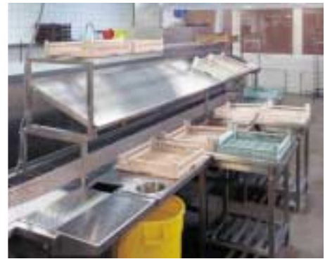
Correctly dimensioned working stations improve ergonomics, speed up working and reduce fatigue. Cutlery soaking works with a lift handle.
