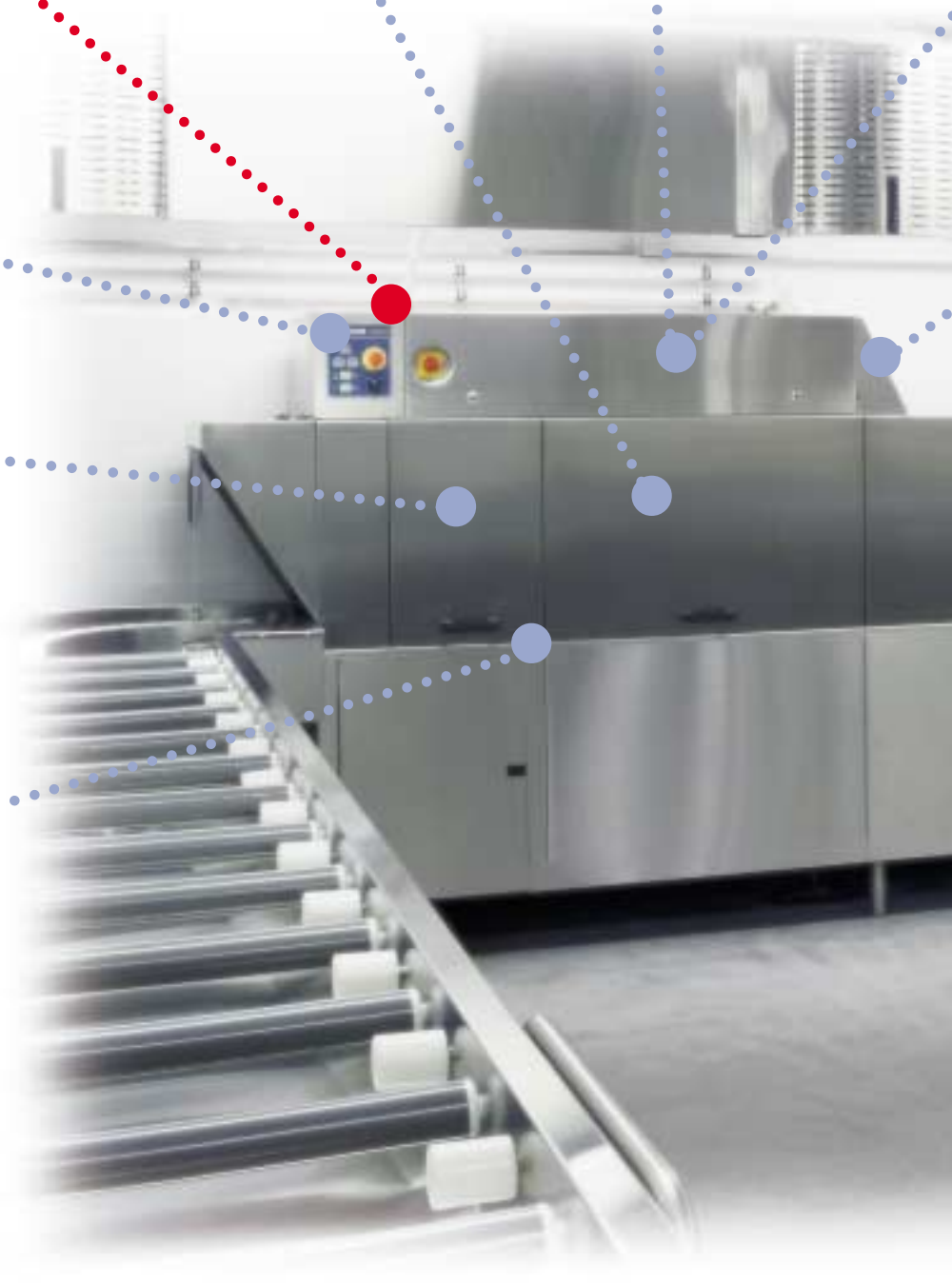
The back wall is neat and solid. All water connections are above the housing. Since all service and maintenance operations can be performed from the front, the machine can be placed almost flush to the wall.
