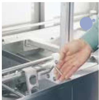
All tanks are drained with one lever. All bottom valves and the overflow pipe close automatically when the rinse zone door is closed.
