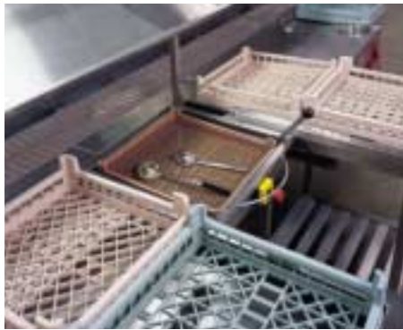
Flight-type dishwashing system equipment with returning and sorting unit in Myllypuro. Two working stations in sorting enable flexible pacing.
