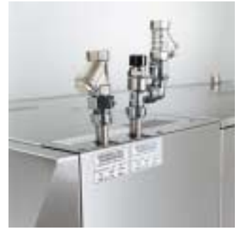
The back wall is neat and solid. All water connections are above the housing. Since all service and maintenance operations can be performed from the front, the machine can be placed almost flush to the wall.
