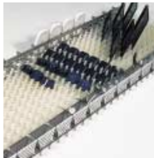
Special belt with cutlery baskets for flight trays, casseroles, cups dishes and cutlery.
