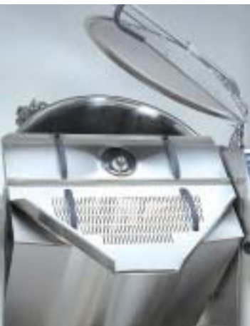
Two-part strainer (300 l). Additional part is used when necessary.
