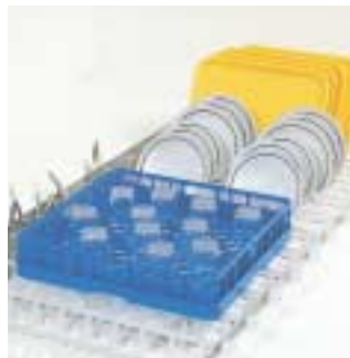
Recessed finger belt with cutlery baskets for trays, flat and deep plates, cutlery and racks with glasses or mugs.
