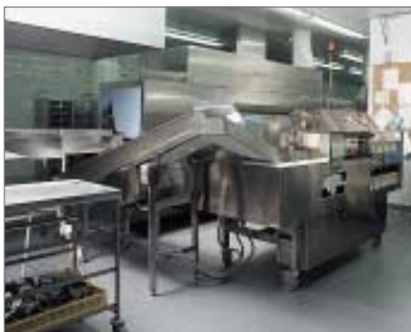
Cutlery dishwasher and sorter comprise a system where washing and sorting to cutlery boxes take place without touching the cutlery.
