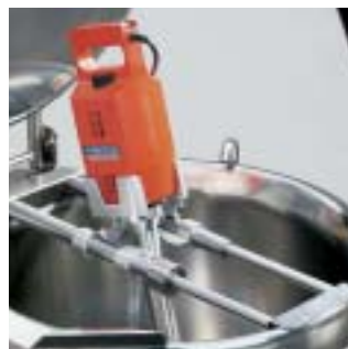
For heavy or lengthy activities the optional kettle support makes working easier.
