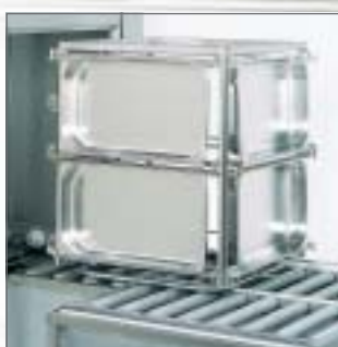
The cassette slides easily on the large rollers on the scraping and loading table.
