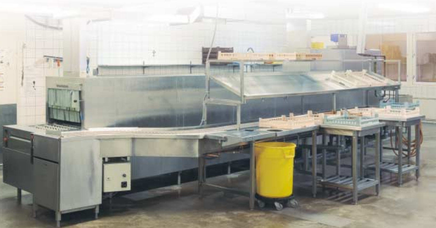
Flight-type dishwashing system equipment with returning and sorting unit in Myllypuro. Two working stations in sorting enable flexible pacing.
