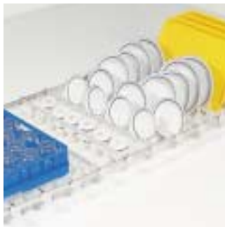
Standard belt with recessed fingers intended for flat and deep plates, cups and trays. Also suitable for racks.
